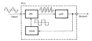
**BLOCK DIAGRAM OF PHASE LOCKED LOOP**
